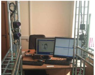
Figure 1: Four camera 3D acquisition system.
