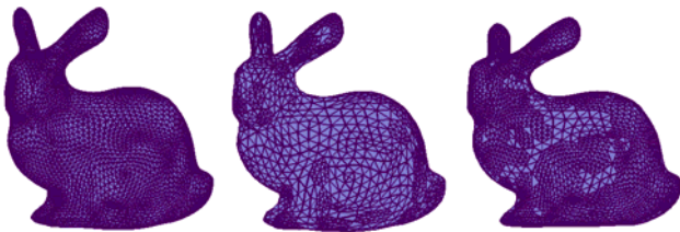
Figure 13: From left to right: respectively full subdivision, adaptive subdivision with an accuracy of 0.1, adaptive subdivision with an accuracy of 0.05.
