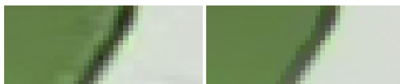
Figure 16: Blind image deringing. Left image: original image with ringing effect, R_E = 1.40 . Right image: the result of automatic deringing with ringing level control, R_E = 1.18 .
