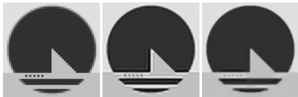
Figure 15: Ringing estimation for image deringing after resampling. Left image: source image upsampled by pixel replication, R_E = 1.05 . Middle image: image interpolated by regularization-based method with low regularization [17], R_E = 1.40 . Right image: interpolated image postprocessed by deringing after resampling, R_E = 1.06 .
