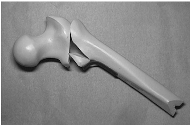
Figure 1: Fractured synthetic bone.
