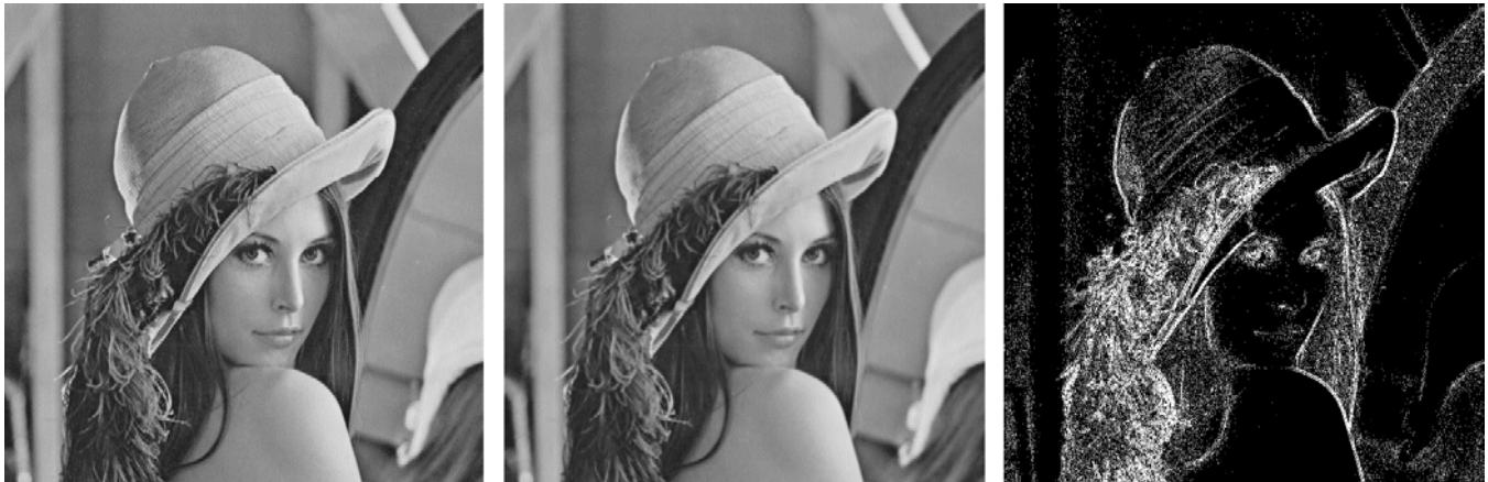
Original (left), blurred “Lena” image, and visualization of the Visible Error Map (right).
