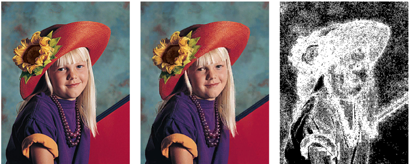
Original (left), 12 times compressed “Portrait” image, and visualization of the Visible Error Map (right).
