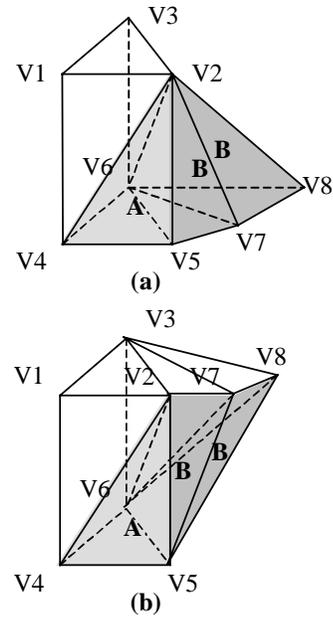
Figure 10: Tetrahedron insertion. In (a), we add two T1-tetrahedrons  $V_5V_6V_7V_2$ ,  $V_7V_6V_8V_2$  to polyhedron  $V_1V_2V_3V_4V_5V_6$  while in (b) we add two T0-tetrahedrons  $V_2V_7V_3V_6$ ,  $V_7V_8V_3V_6$  and one T2-tetrahedron  $V_5V_6V_8V_7$  to it.
