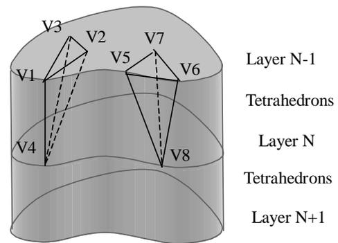
Figure 3: A layered tetrahedron model. Tetrahedron  $V_1V_2V_3V_4$  and  $V_5V_6V_7V_8$  are called non-border (internal) tetrahedron and border tetrahedron respectively if the former does not include the model's surface facet while the latter does.
