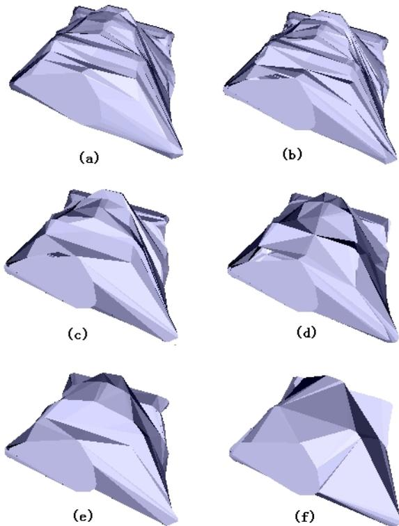
**Figure 11:** Simplified models with different simplification rate. (a) is the original model; (b), (c), (d), (e), (f) is the simplified ones with simplified rates of 50%, 75%, 90%, 95%, 99% respectively.
